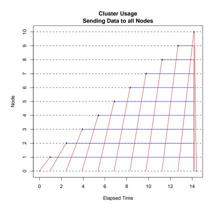
Figure 2: Visualization of timing information for cluster usage for component test 1 with the **snow** package using MPI. Green rectangles (near the diagonal) representing active computation (in this case very small), blue horizontal lines representing a worker waiting to return a result, and red lines representing master-slave communications.
