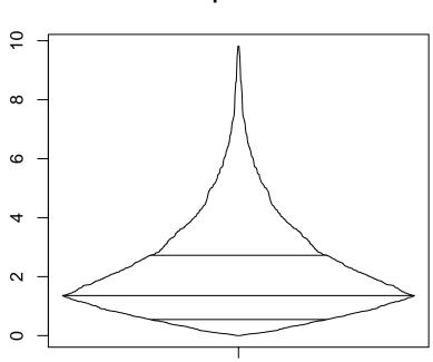
Figure 5: A box-percentile plot showing the typical pattern for skewed distributions. Compare this plot to the box-percentile plot for normal data with outliers shown in Figure 4.
