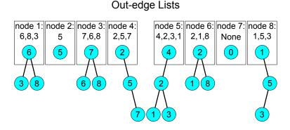
Figure 3: This is one possible **ergm** representation of the out-edges for the network of Figure 2. The network would be redundantly represented as a set of in-edge trees.
