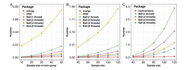
Figure 7: Runtime analysis for **energy**, **multivariance**, **HHG**, and **Ball** in the K-sample test and test of (mutual) independence problems in metric spaces. A) the K-sample test problem (K = 4), B) the test of independence problem, C) the test of mutual independence problem. The runtimes (y-axis) are measured in seconds.
