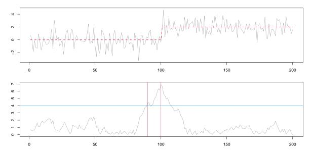
Figure 2: Top: A time series with one mean changes at the location 100, where the underlying step signal  $f_t$  is overlaid as dashed line. Bottom: The corresponding absolute MOSUM detector  $|T_G(k)|$  for k = 1, ..., n with bandwidth G = 20. The critical value for level  $\alpha = 0.05$ is denoted by a horizontal line, and maximal points within significant environments of  $T_G(k)$ are highlighted by the vertical lines.
