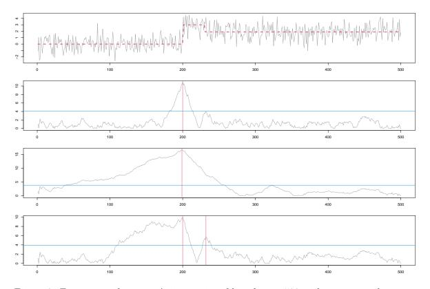
Figure 6: From top to bottom: A time series of length n = 500 with two mean changes at the locations 200 and 230 of respective height 3 and -1.1, and the corresponding absolute MOSUM detector  $|T_{\mathbf{G}}(k)|$  for k = 1, ..., n with (symmetric) bandwidths G = 30, 120 and  $\mathbf{G} =$ (30, 120). Critical value at level  $\alpha = 0.05$  is visualized by a solid horizontal line and the change-points estimated according to the  $\eta$ -rule by solid vertical lines.
