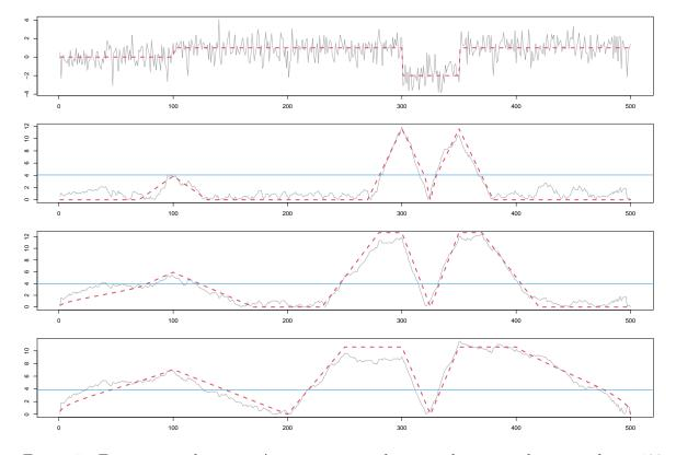
Figure 5: From top to bottom: A time series with mean changes at locations  $k_1 = 100$ ,  $k_2 = 300$  and  $k_3 = 350$ , where the underlying step signal  $f_t$  is overlaid as dashed line, and the absolute MOSUM detector  $|T_G(k)|$  for G = 30,70 and 100, where the absolute MOSUM signal  $|T_G(k; f)|$  is overlaid as dashed line and the critical value at level  $\alpha = 0.05$  is visualized by a solid horizontal line.
