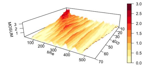
Figure 10: Surface plot visualization of the MOSUM detectors computed with a range of bandwidths on a realization of the mix test signal from Section 3.1.
