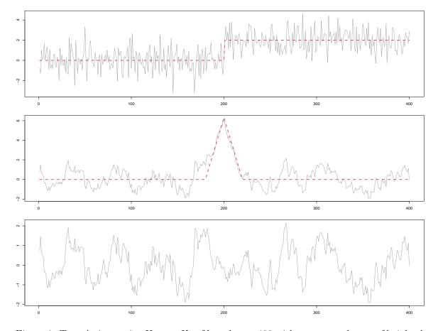
Figure 1: Top: A time series  $X_1, \ldots, X_n$  of length n = 400 with one mean change of height d = 2 at time k = 200. The corresponding step signal  $f_t$  is overlaid as dashed line. Middle: The MOSUM detector  $T_G(k; X)$  for  $k = 1, \ldots, n$ , where the MOSUM signal  $T_G(k; f)$  is overlaid as dashed line. Bottom:  $T_G(k; e) = T_G(k; X) - T_G(k; f)$ .
