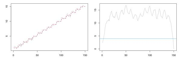
Figure 4: Left: A time series of length 150 with mean changes at locations 10, 20, ..., 140, where the underlying step signal  $f_t$  is overlaid as dashed line. Right: The corresponding scaled absolute MOSUM detector  $\sigma^{-1}|T_G(k)|$  with G = 15; the critical value for level  $\alpha = 0.05$  is denoted by a horizontal line. The series is a realization of the model stairs10 from Fryzlewicz (2014) (see Section 3.1).
