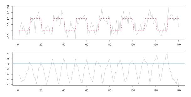
Figure 3: Top: A time series of length 140 with mean changes at locations 10, 20, ..., 130, where the underlying step signal  $f_t$  is overlaid as dashed line. Bottom: The corresponding scaled absolute MOSUM detector  $\sigma^{-1}|T_G(k)|$  with G = 8; the critical value for level  $\alpha = 0.05$  is denoted by a horizontal line. The series is a realization of the model teeth10 from Fry-zlewicz (2014) (see Section 3.1).
